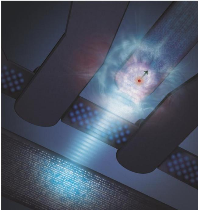
Artist's impression of a phosphorus atom (red sphere surrounded by electron "cloud", with arrow showing the spin direction) coupled to a silicon single-electron transistor. A burst of microwave radiation (light blue) is used to 'write' information on the electron spin.
